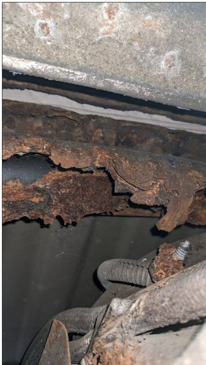
Failed frame cross-member on Eric's truck
